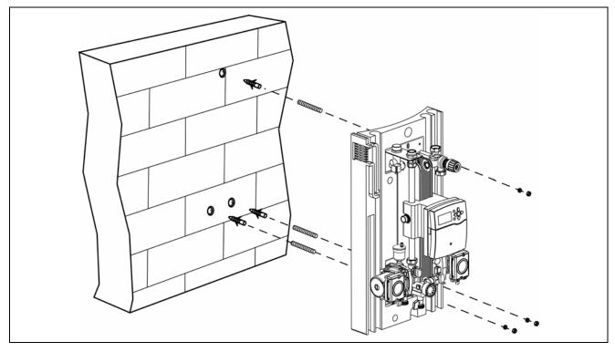
Wall installation takes place as follows with the included attachment material (3x M10 stair bolts, M10 nuts and 3 M10 washers):
